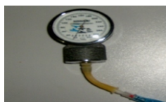
Figure 1: Pressure gauge adapted to the end of an infusion set to verify the cuff pressure.
