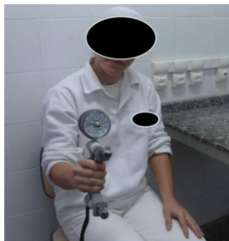
Figure 3 - JAMAR® dynamometer. - Source: (REIS AND MORO, 2012).
