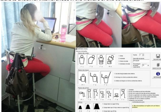
Figure 2 - Layout seat and bench for use at the desk next to OWAS analysis by Ergolândia software 5.0 trial version
