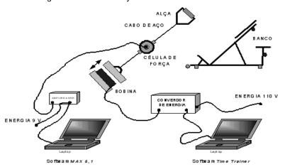
Figure 1 Illustrative scheme of the data collecting system. Proceedings
