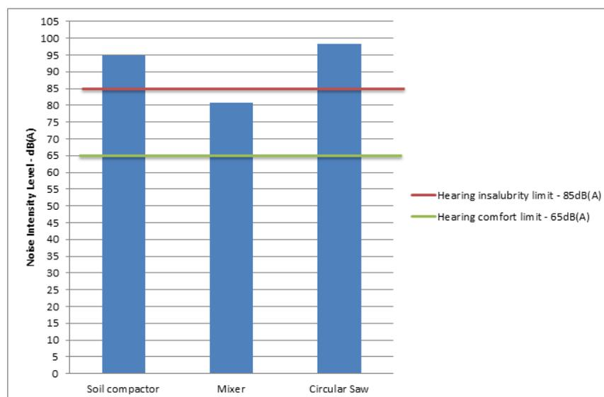
Figure 1 - Noise values obtained for the three workstations analyzed and compared with the limit for unhealthiness, 85 dB (A), according to the NR-15.
